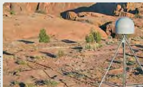
A backbone network of 116 new and 20 existing GPS receivers provide a long-wavelength, long-period synoptic view of the entire plate boundary zone, including the eastern U.S.
