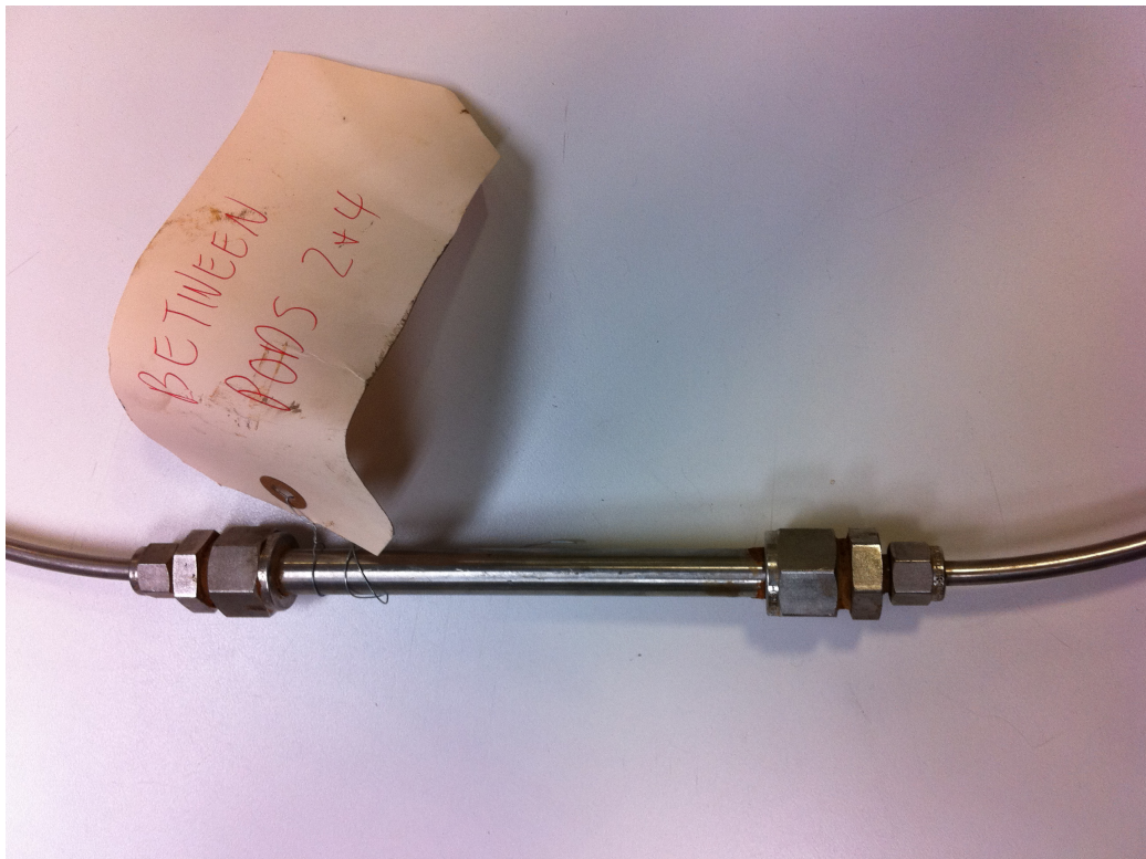
Figure 9 Splice Housing Between Pods 2 and 4
