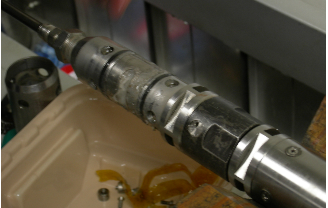
Figure 10E Cable in Upper Left Corner Connected to Instrument Housing in Lower Right Corner Through Cable Head in Center.
