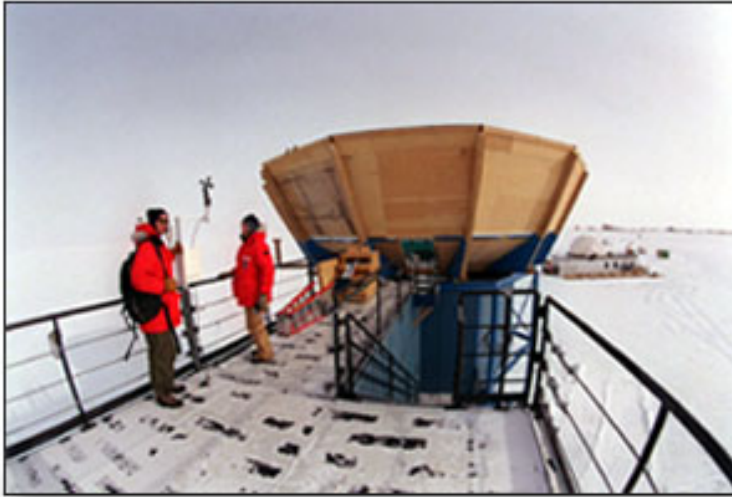
Scientists stand outside the Degree Angular Scale Interferometer (DASI), the microwave detector at the Amundsen-Scott South Pole station on 6 January 2001. The detector was used by University of Chicago scientists and others to detect microwave evidence of the Big Bang in which the universe was thought to be created about 14 billion years ago.
