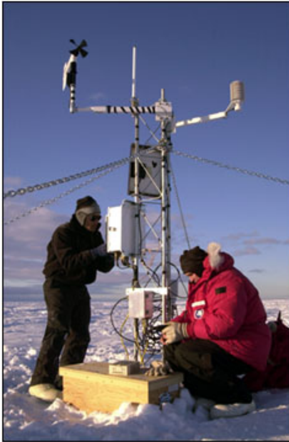
Johnathan Thom (in black) of the University of Wisconsin at Madison and Doug MacAyeal (in red) of the University of Chicago install on the large tabular iceberg B-15A a tower with instruments that will relay position, temperature, wind speed, pressure and humidity to a satellite. Scientists will be able to track the conditions on and around the iceberg as it makes its way through the waters of Antarctica. (NSF photo by Josh Landis)
