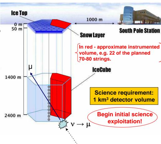
IceCube will occupy a volume of one cubic kilometer. Here we depict one of the 70-80 strings of optical modules (number and size not to scale). IceTop located at the surface, comprises an array of sensors to detect air showers. It will be used to calibrate IceCube and to conduct research on highenergy cosmic rays.
