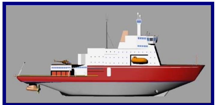
Fig. 8: Outboard profile of the PRV showing dual podded propulsors although traditional line shafting remains an alternative
