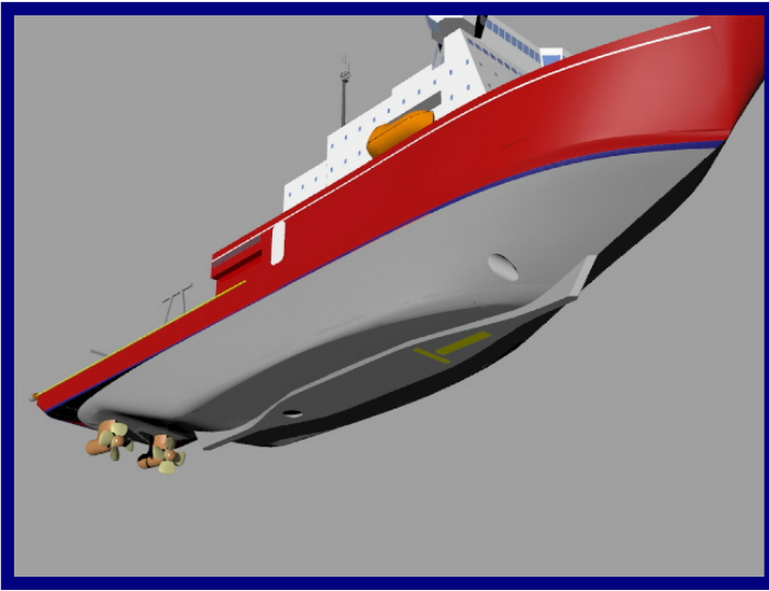
Fig. 2: Underwater view of PRV box keel with bottom mapping sensors
