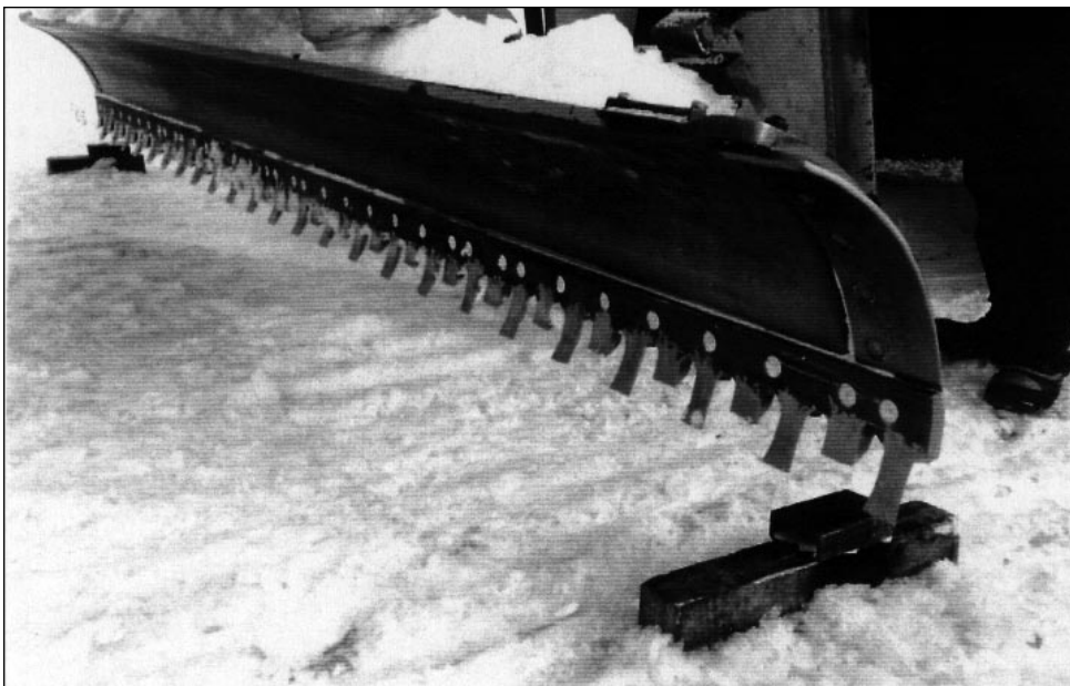
Figure 3. Custom-built grader blade for leveling glacial ice.
