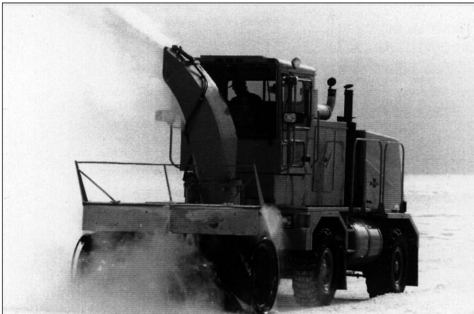
Figure 4. Large-capacity snowblower used to remove snow and graded ice from runway.
