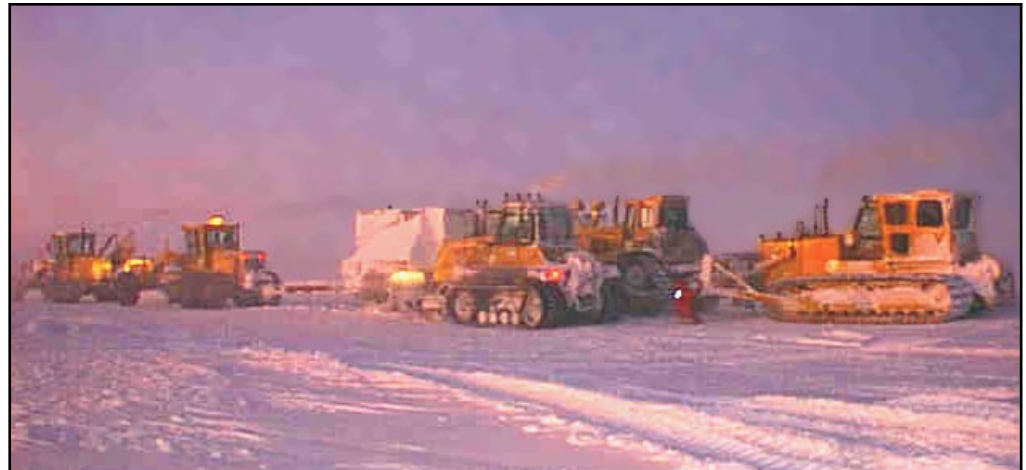
The road grader pulls the proof cart to prepare the Pegasus blue-ice runway for winter fly-in landings.
