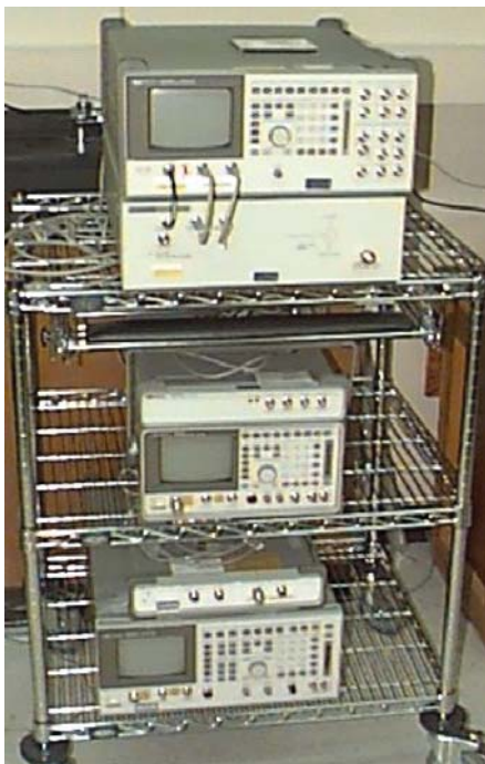
Base station simulators
