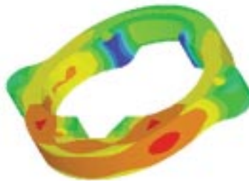
Virtual manufacturing research includes finite element analysis for preprocess determination of manufacturing errors related to geometrical accuracy and thermal variations due to machines and environment. Shown is a graphically represented analysis for a gear pump housing.
