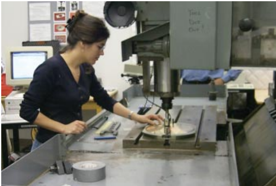
Students receive practical metrology experience. Here a student uses a grid encoder to investigate the dynamic errors of a machining center.
