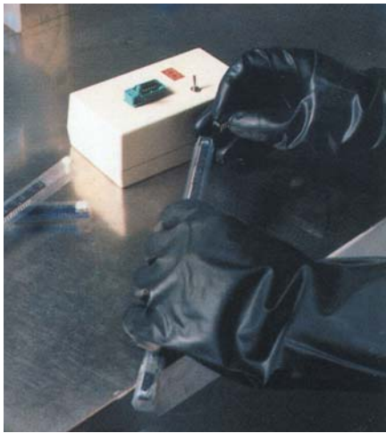
The Static Bug: This innocent looking “spy” chip is being loaded into product wafer carriers for shipment to the customer. Upon receipt, the customer will insert the chip into a test fixture to determine if a previously established electric field intensity has been exceeded.
