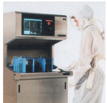
Tencor Instruments used CMC light scattering technology to obtain improved performance in the Surfscan 6400.
