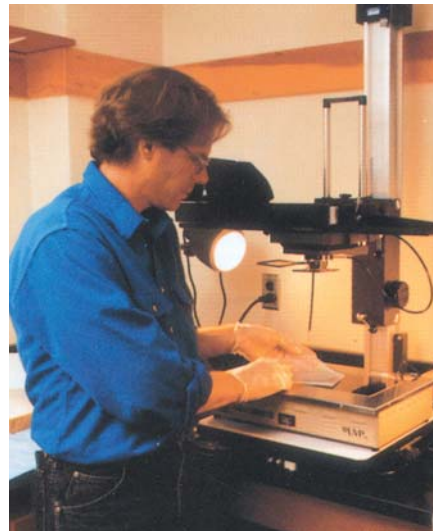
Microbiologist Mark Burr prepares to stain amplified DNA with ethidium bromide to measure the bacterial content of ultrapure water used to process semiconductor wafers. This process, developed by Professor Ian Pepper, promises to revolutionize microbial water metrology.
