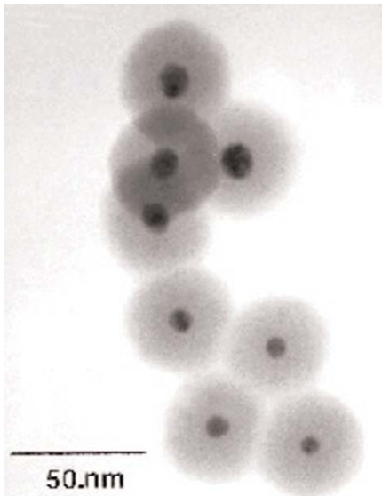
TEM of nanocomposite Silver core/silica shell particles.
