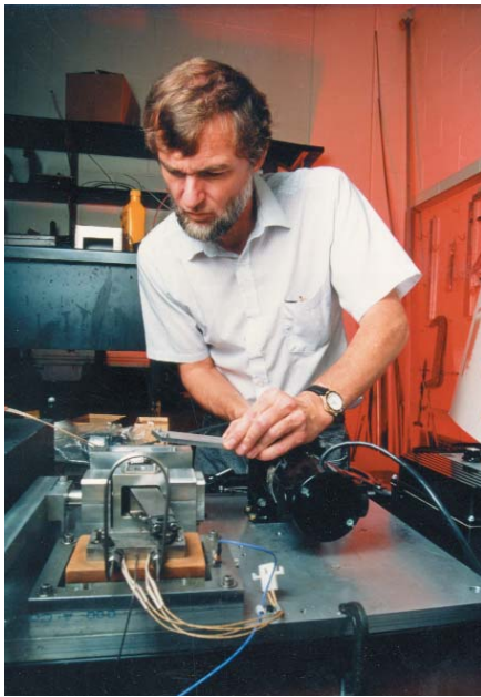
Dr. Scott Bair adjusting a custom reciprocating tribosimulator.
