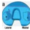
Page 10 Comparison of experimental and simulated wear regions for total knee replacement design after 5 million cycles of walking performed in a knee simulator machine. Credit: B.J. Fregly, University of Florida
