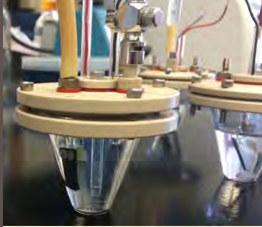
▲ Many bioreactors used for growing microorganisms with electrodes.
