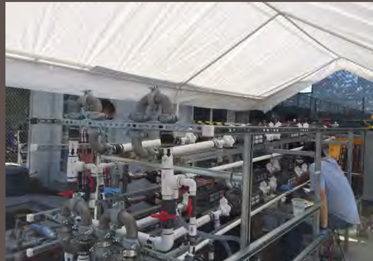
▲ Bacteria, archaea and single cell eukaryotes are extremely important to industrial applications including wastewater treatment. The picture shows a large-scale microbial fuel cell installation treating swine waste at the Escondido high school agriculture center.
