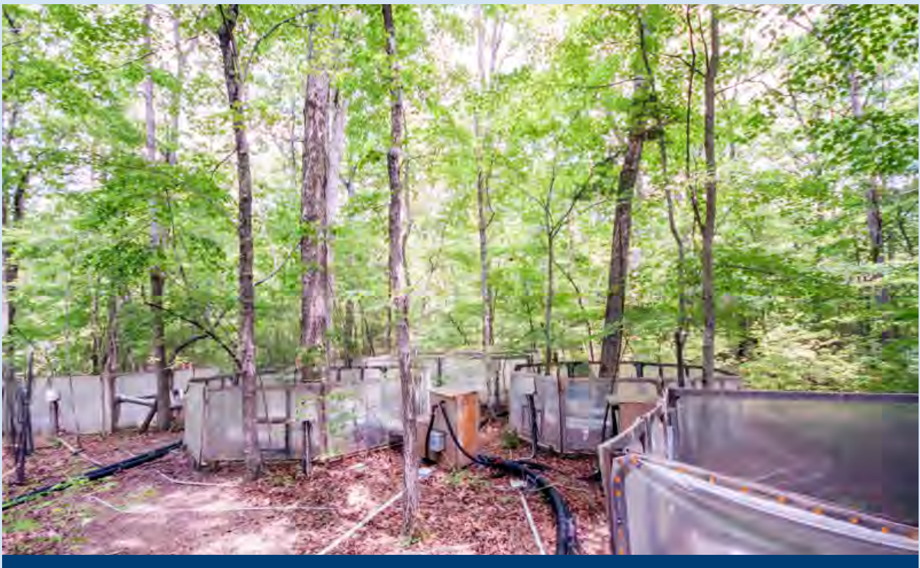
^ Open-top chambers at the Duke Forest site in North Carolina. Built in 2009 at sites in both North Carolina and Massachusetts, the warming chambers consist of 12 open-top warming chambers, nine of which are pumped with warm air to simulate predicted global warming.
